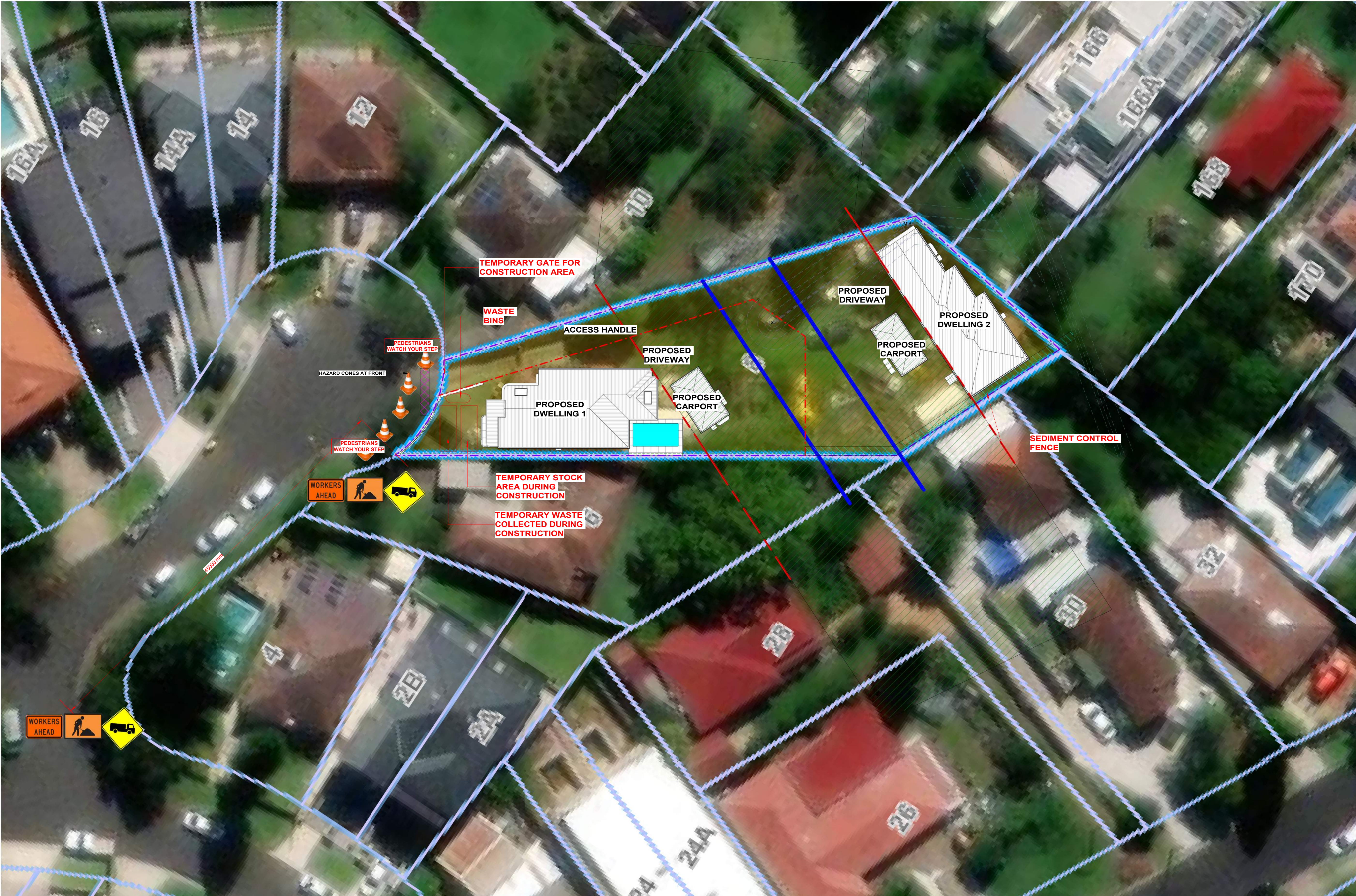
1 CONSTRUCTION, TRAFFIC & WASTE MANAGEMENT PLAN 1 : 200
